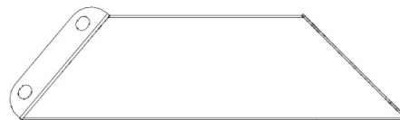
D03 CORBEL - A4M01826 (x1) 2 3/4"x5 11/16"x20 1/16" (70x145x509)
