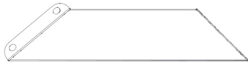
D06 CORBEL - A4M01832 (x1) 2 3/4"x5 7/8"x24 13/16" (70x149x631)
