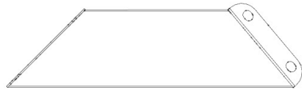
D04 CORBEL - A4M01830 (x1) 2 3/4"x5 11/16"x20 1/16" (70x145x509)
