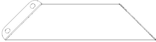
D02 CORBEL - A4M01818 (x1) 2 3/4"x5 13/16"x22 1/4" (70x147x565)
